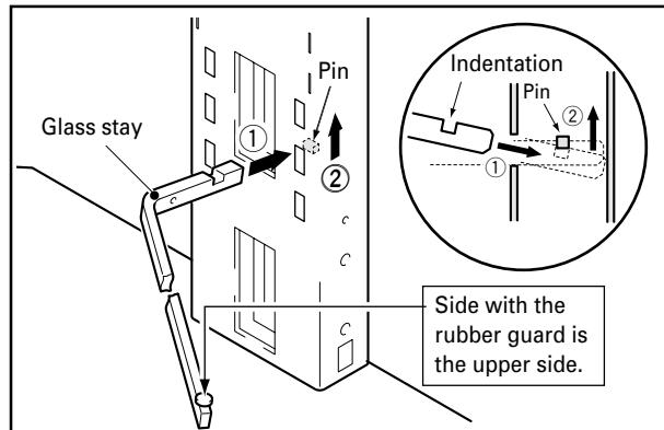
Glass stays may be inserted into the upper, middle, or lower holes to adjust the height of the glass panel (The middle holes are designed to be used for standard installation).
