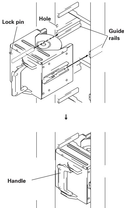
Shown above is the insertion to the front magazine bay. Though the insertion to the rear magazine bay is almost same but note that the proper installation position is in the place where it is very secluded.
