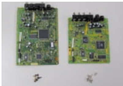
Main substrate unit and screws using no lead or hexavalent chromium (right) and the conventional items (left)
