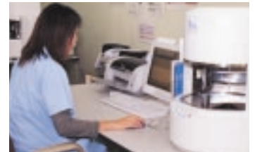
Using a fluorescent X-ray analyzer for detailed examination of hazardous content in products
