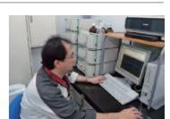
Measuring VOCs using a high-performance liquid chromatograph (HPLC) analyzer
