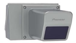
[3D-LiDAR "1st Model" (Medium Range)]
