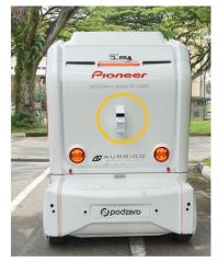
[Autonomous shuttle bus with Pioneer's 3D-LiDAR sensor]
