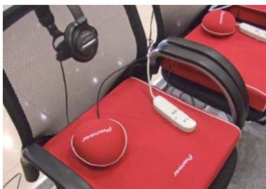
The "Listen through the Body" vibrating acoustic system transmits realistic musical vibrations directly to the listener's body through seat cushions and a small pouch with built-in vibration units.
