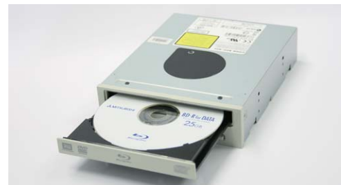
● Pioneer is developing a disc drive product compatible with BD-R discs with organic dye/metal nitride recording layers. Shown here is a prototype displayed at CEATEC JAPAN* 2007.
